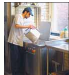
Manual feeding of MV-180 freestanding bench inlet
