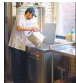
Manual feeding of MV-180 freestanding bench inlet
