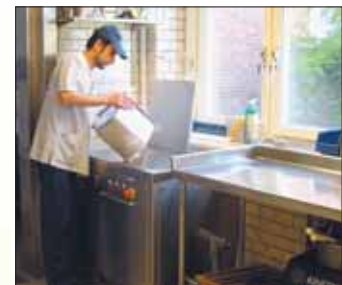
Manual feeding of MV-180 freestanding bench inlet
