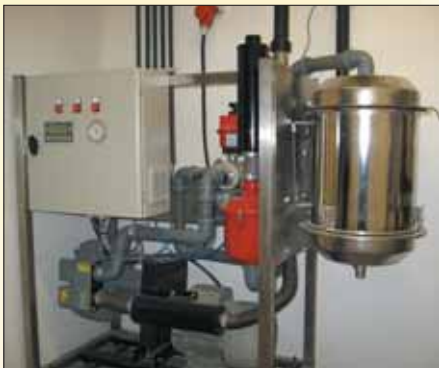
MV-7.5 vacuum pump and PLC control module
