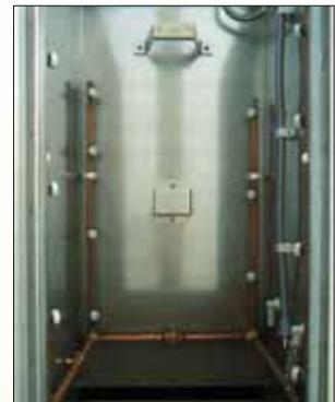
High pressure nozzles for hot water rinsing of sleeve
